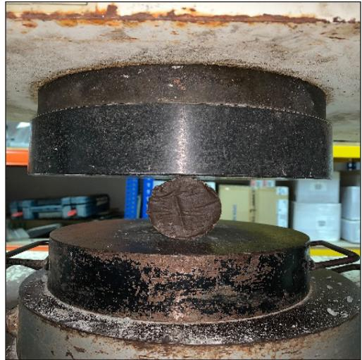
Figure 7. Splitting tensile test
