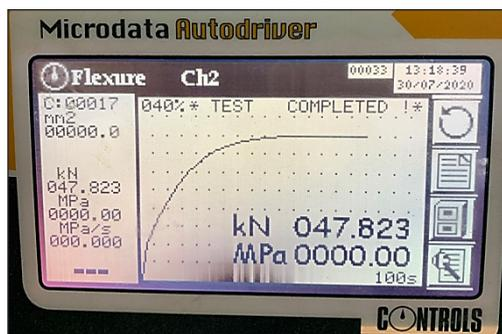
Figure 10. Flexural tensile machine (Microdata control flexure)
