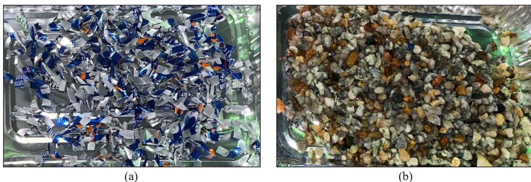
Figure 2. (a) Sample of cut waste tin fibre; and (b) Sample of twisted tin fibre
